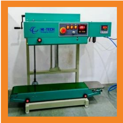
Nitrogen Flushing Machine
